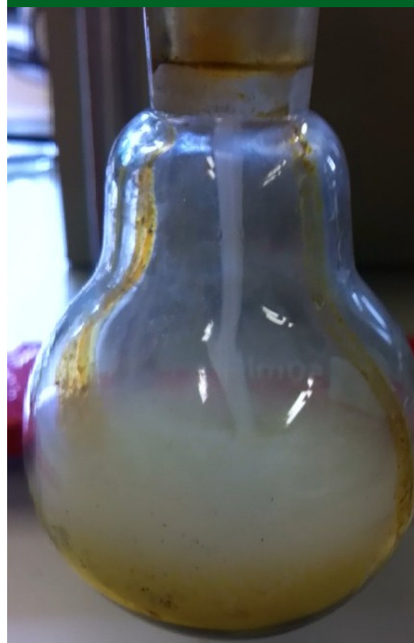
Figure 2: Formation of bio-oil from the electrostatic precipitator.
